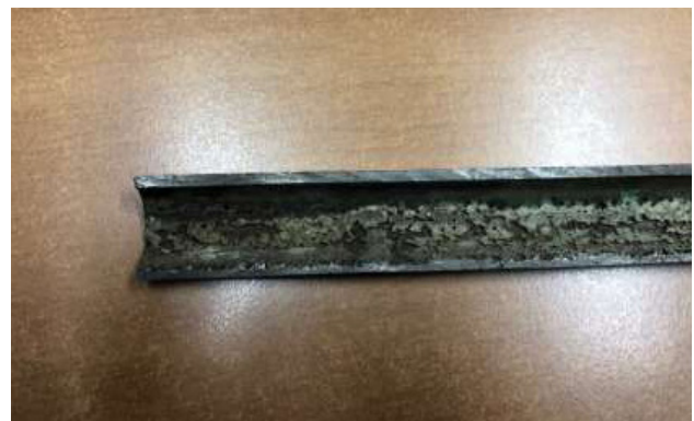
Figure 2: Cut U-tube with wall loss.
