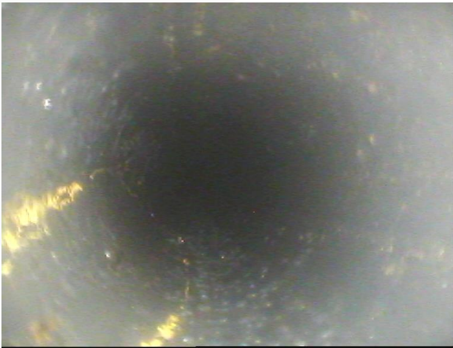
Fig 4: Wall loss at 6m in R[7]C[18]
